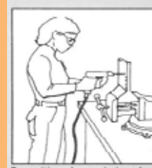
Reposition clamped piece for ideal drilling position.
