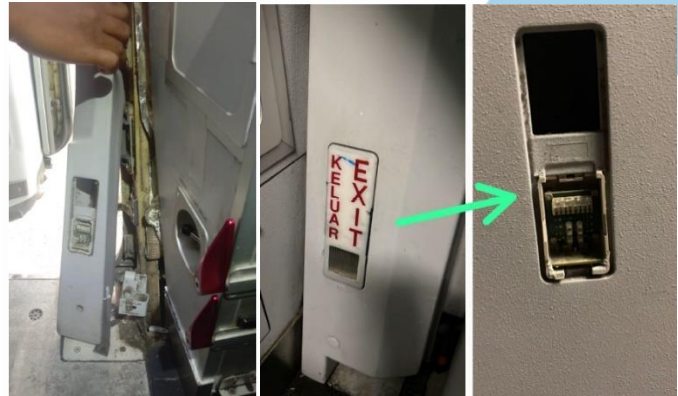
Gambar 2. Aft Emergency Exit Light (RH Side) Not Illuminate
