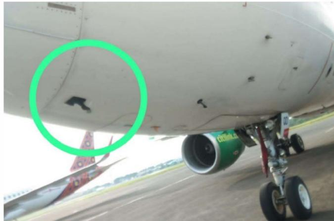
Gambar 1. Kondisi Damage Post Incident
