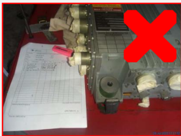
Example of EEC (Electronic Engine Control) Placed on Tool Drawer and Covered by Tape
