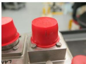
IMPROPER WIRELOCKING ATTACHED (PROPER TYPE SHOULD BE BERGEN SAFETY CABLE)
