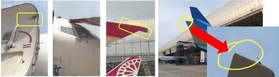
Gambar 1. Contoh Kasus Friction/Collision saat Towing atau Pushback (for Internal Purpose Only)
