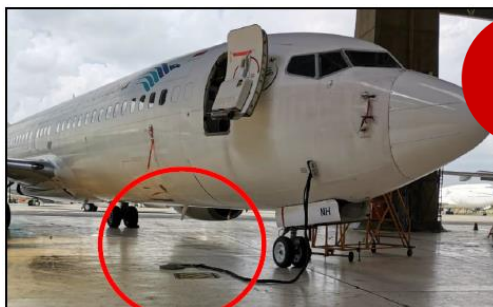
Ground Power Port without safety cone
