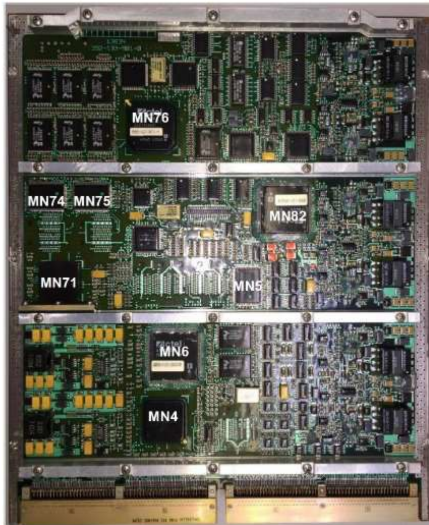
Picture 1. EEC electronic board, MN4 location
