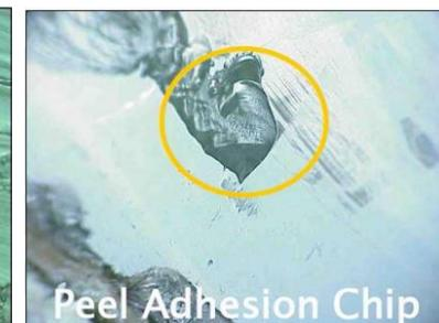
*Peel Adhesion Chip*
