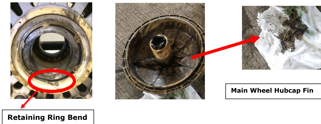
Gambar 1. Main Wheel Hubcap fin no. 2 damage and retaining ring bend
