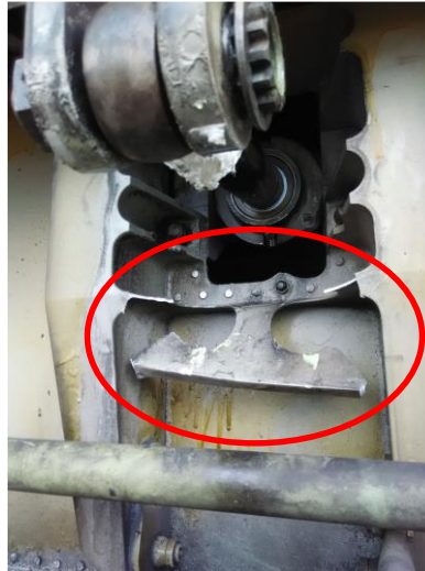
Gambar 1. Spoiler #8 B747-400 Fitting Damage
